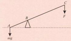
A lever consists of a uniform steel rod AC of weight 100 N and length 2k m, which rests on a pivot at B that has a height of 0.3k m. AB = 0.5k m. A mass m kg is attached to the lever at A. The mass is lifted by means of a force of magnitude FN that is applied vertically downwards at C. Show that  $F > \frac{1}{3}(mg - 100)$ .
