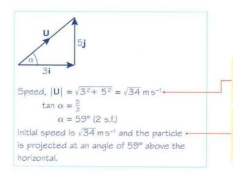
Speed is the magnitude of the velocity vector. If the initial velocity is  $p\mathbf{i} + q\mathbf{j}$  m s<sup>-1</sup>, the initial speed is  $\sqrt{p^2 + q^2}$ .
