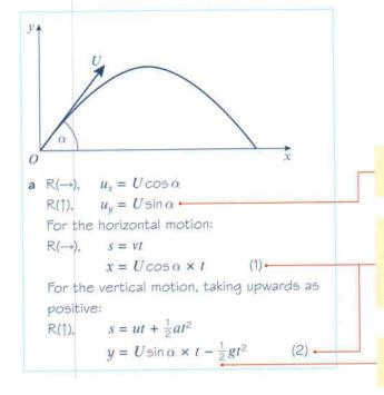
Resolve the velocity of projection horizontally and vertically.
