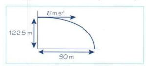
Projected horizontally,  $R(\rightarrow)$ ,  $u_x = U$  Taking the downwards direction as positive,  $R(\downarrow)$ ,  $u_y = 0$   $R(\downarrow)$ , u = 0, s = 122.5, a = 9.8, t = ?  $s = ut + \frac{1}{2}at^2$   $122.5 = 0 + \frac{1}{2} \times 9.8 \times t^2$   $122.5 = 4.9t^2$   $t^2 = 25$  so t = 5  $R(\rightarrow)$ , v = U, s = 90, t = 5 s = vt  $90 = U \times 5$   $U = 90 \div 5$  so  $U = 18 \, \mathrm{m \, s^{-1}}$
