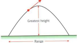
A projectile reaches its point of greatest height when the vertical component of its velocity is equal to 0.
