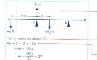
Draw a diagram showing the forces. Remember, as the beam is 'on the point of tilting', C is a pivot and the reaction force at D is zero.
