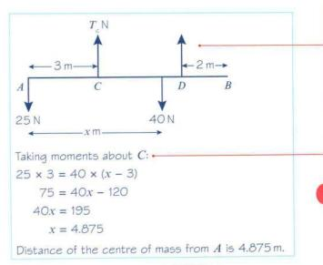
Draw a diagram showing the forces about C. As the rod is 'on the point of rotating', C is a pivot and the tension force at D is zero. As the rod is non-uniform you don't know the distance from A to the centre of mass, so you can label it as x.
