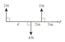
4 The diagram shows a set of forces acting on a light rod. The resultant moment about P is 12.8 Nm clockwise. Find the value of x.
