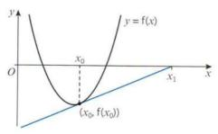
Because  $x_0$  is close to a turning point the gradient of the tangent at  $(x_0, f(x_0))$  is small, so it intercepts the x-axis a long way from  $x_0$ .
