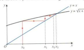
Read up from  $x_0$  on the vertical axis to the curve  $y = \sqrt{x+1}$  to find  $x_1$ . You can read across to the line y = x to 'map' this value back onto the x-axis. Repeating the process shows the values of  $x_n$  converging to the root of the equation  $x = \sqrt{x+1}$ , which is also the root of f(x).
