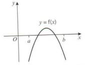
There are multiple roots within the interval [a, b], but a sign change does not occur. In this case there is an **even number** of roots.
