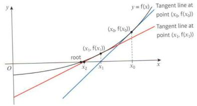
If the starting value is not chosen carefully, the Newton–Raphson method can converge on a root very slowly, or can fail completely. If the initial value,  $x_0$ , is near a turning point or the derivative at this point,  $f'(x_0)$ , is close to zero, then the tangent at  $(x_0, f(x_0))$  will intercept the x-axis a long way from  $x_0$ .
